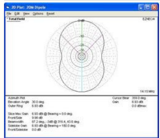
Figure 1: Azimuth pattern of a half-wave dipole at a height of half a wavelength has a -3 dB beamwidth of of 87 degrees on each side -- a close match to the coverage needed by W1ZR to reach US and Canadian stations.
