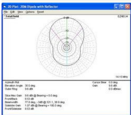
Figure 2: By adding a 5 percent longer than the dipole and 6 feet behind it, I reduce -- but don't eliminate -- rearward radiation and provide some gain to the front where distances are longer. (for bigger picture see ARRL website)
