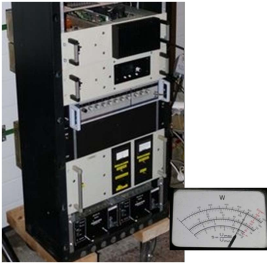
Figure 19. Beacon transmitter, capable of 850-W RF output continuous transmission at 5.39 MHz.
